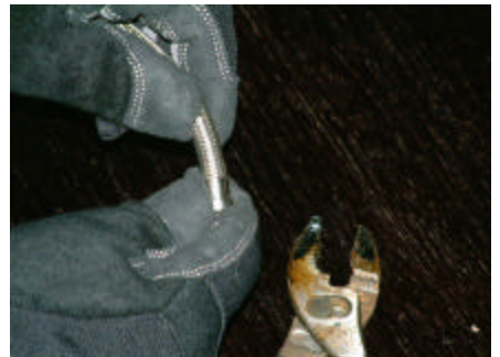
Now that you have the braid in the ferrule twist the ferrule over the hose.
