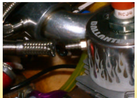
Now take your completed Hose Assembly and slide it onto your existing barb fittings. If hose I.D. is too small you can drill the inside of the hose to fit.
