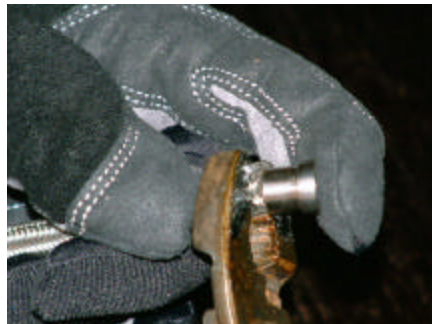
Use a pair of pliers to compress the braid so it will fit in the ferrule. You will need to make sure not many braids stray to the outside of the ferrule. Use slight pressure to get the ferrule to slide over the braid.
