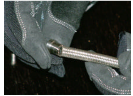
Try to get as much hose in the ferrule. Keep it at an angle and try not to let the braid on the hose start to flare out.
