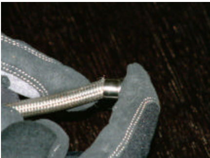
Now that you have as much hose in the ferrule as you can get, apply pressure to the ferrule to hold it in place.
