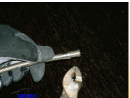
Pull back the ferrule about a half inch. You may need to use your pliers. Now repeat all the steps to the other side.
